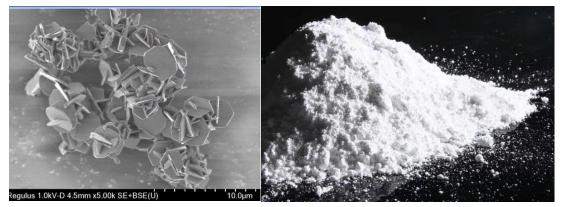
Flake alumina has excellent intrinsic properties and special structural characteristics. Therefore, it has many excellent properties:
