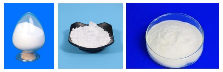
Pseudo boehmite, chemical formula is  $\alpha$  - ALOOH, also known as pseudo monohydrate, is non-toxic, odorless, odorless, white colloid (wet) or powder (dry). It has the characteristics of high purity, good solubility, strong adhesion, high specific surface and large pore volume, and its water state is thixotropic gel.
